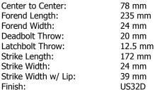
Fasteners: Two (2) 4 mm x 25 mm FPHWS and three (3) 3.5 mm x 20 mm FPHWS
