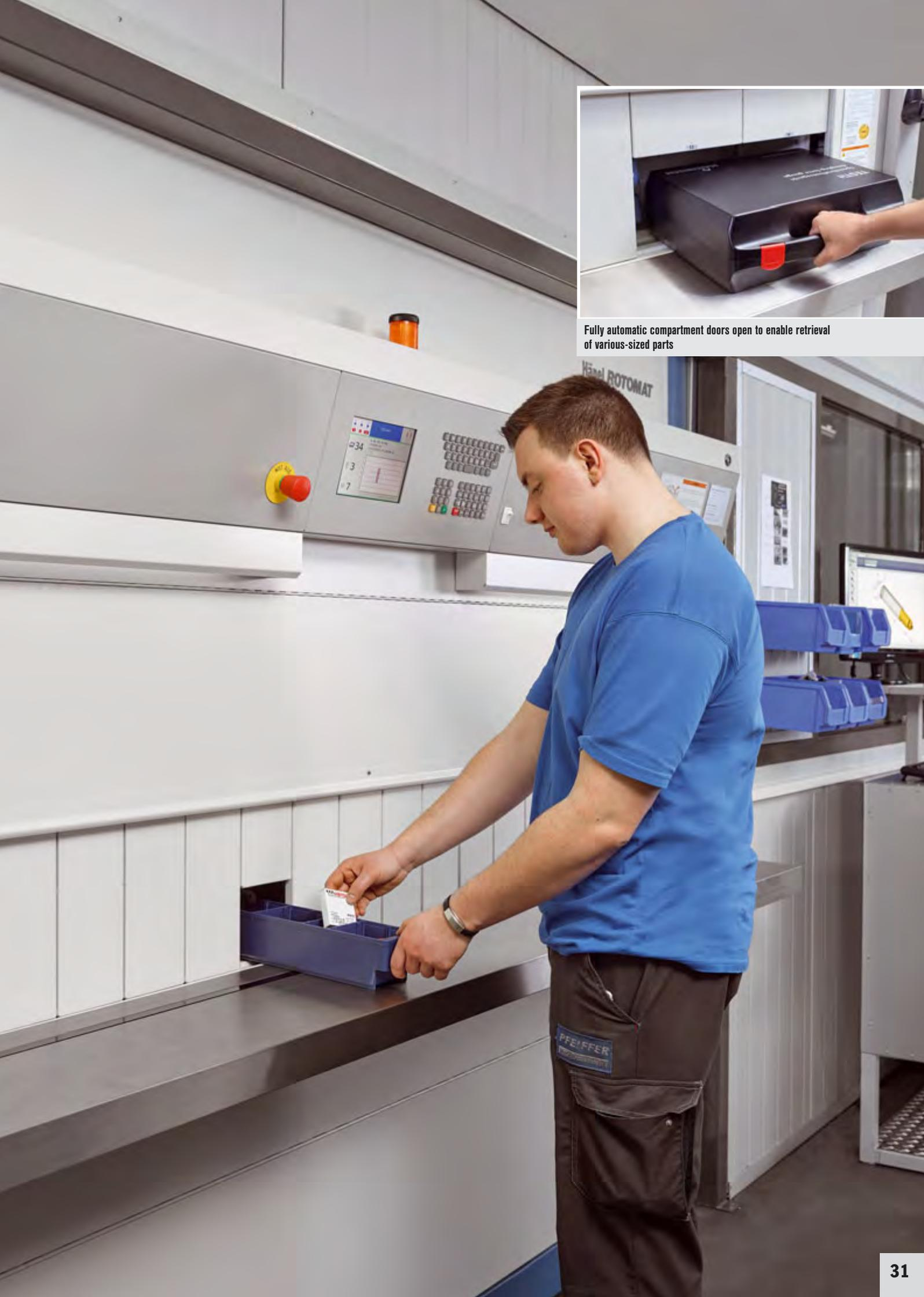
Fully automatic compartment doors open to enable retrieval of various-sized parts
